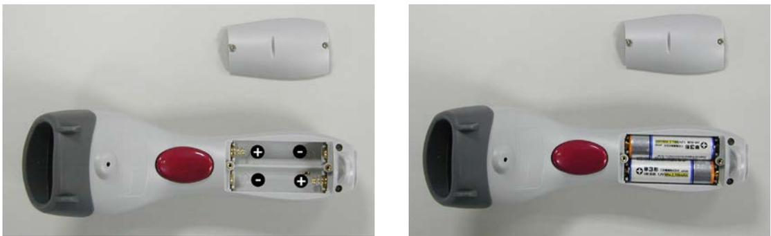
Put back the battery cover, and tighten the screws.
