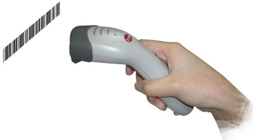
Note that best scanning results are usually obtained by tilting the scanner up or down a little – reflections can affect the scanning performance
