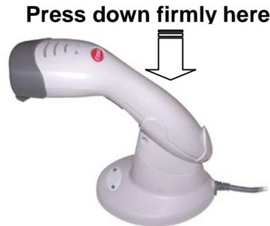
To start charging, press either of the small buttons at the side of LED indicator on the base (as shown below). The red LED on the scanner will light to show that it is being charged.
